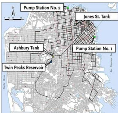
**The auxiliary water supply system (AWSS), constructed after the 1906 earthquake, is a water distribution system operated and maintained by the San Francisco Fire Department. It delivers water under high pressure for fire fighting and is independent from San Francisco's domestic water system. It consists of 2 pump stations, 2 water storage tanks, 1 reservoir, 172 cisterns, and approximately 135 miles of pipes.**
