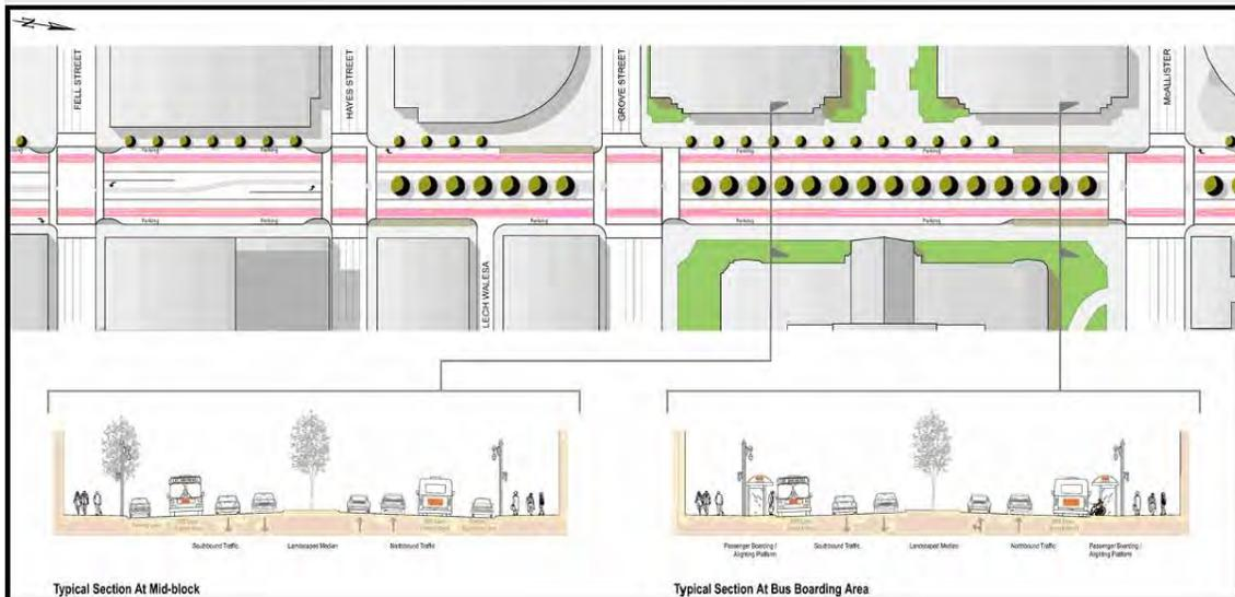
Figure 2.1 Preliminary Plan and Section View of Alternative 2
