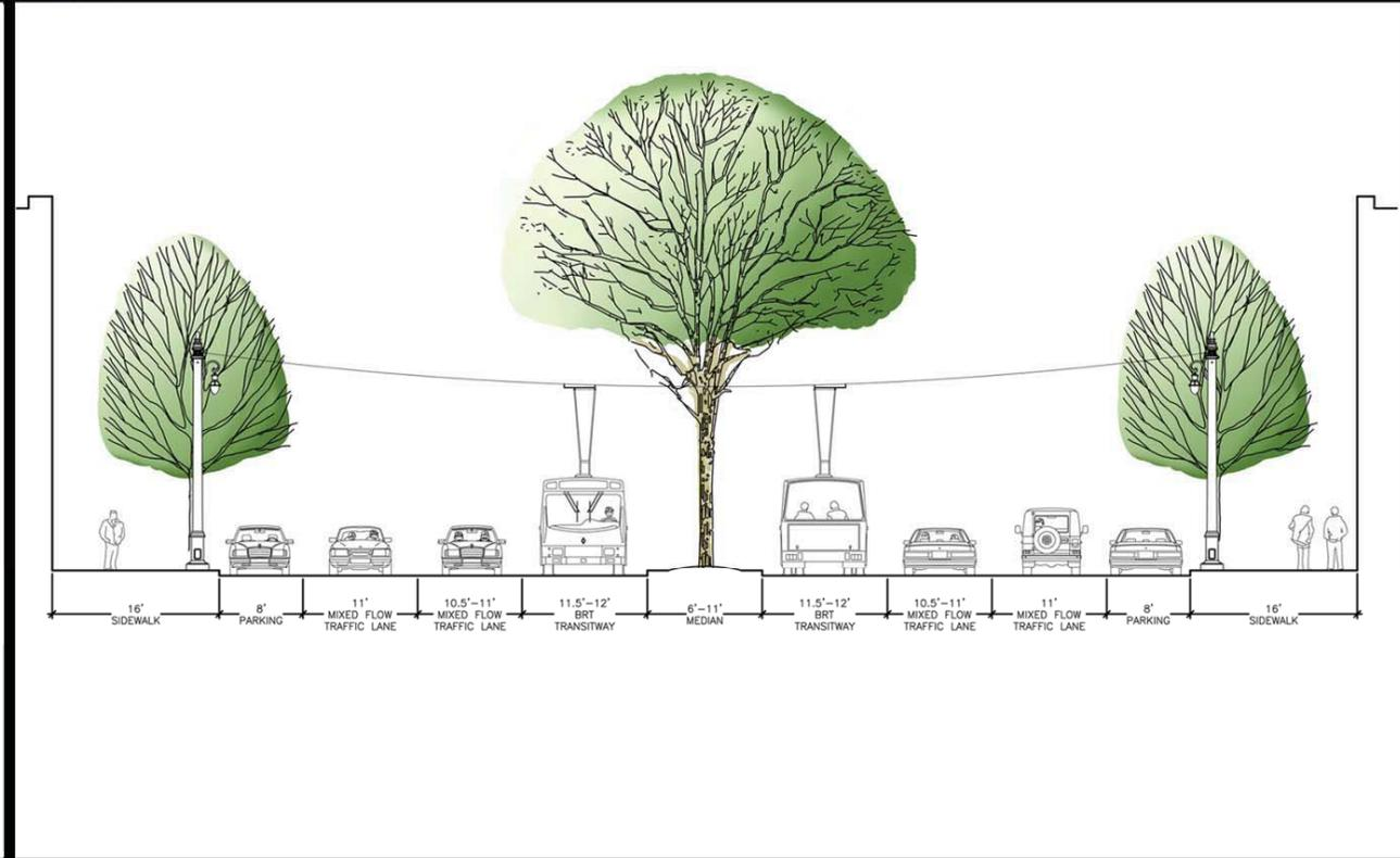
**LPA: Center Lane BRT with Right-Side Boarding/Single Median and Limited Left Turns**
