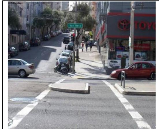
**Figure 9 – Nose Cones Provide a Pedestrian and ADA Refuge when Crossing Van Ness Avenue**
