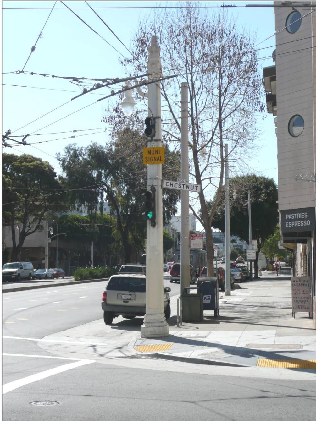
**Photograph 5: Electric traffic signal and MUNI signal equipment inserted and signage added to Pole 287, southwest corner of Van Ness Avenue and Chestnut Street, 4/1/2009.**
