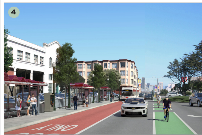
Palm to Broderick (including Masonic): Side Bus Lanes Enables bus improvements while balancing the need for: pedestrian access, security and safety, short transfer (surface stop); smooth multimodal interactions, including new bike lane; accommodating high vehicle volumes. Responds to community feedback preferring surface stop at Masonic.
