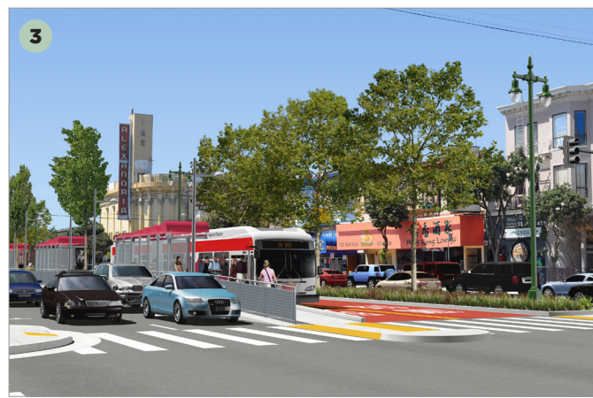
27th Ave to Palm: Center Bus Lanes, Consolidated Local-BRT Stops Provides 30% travel time savings and high reliability with separation from parking and loading. Speeds travel for the most riders—local bus and BRT. Preserves most on-street parking. Installs new medians with lighting and landscaping. Provides pedestrian crossing safety improvements, including bulb-outs and reductions in left-turn conflicts.
