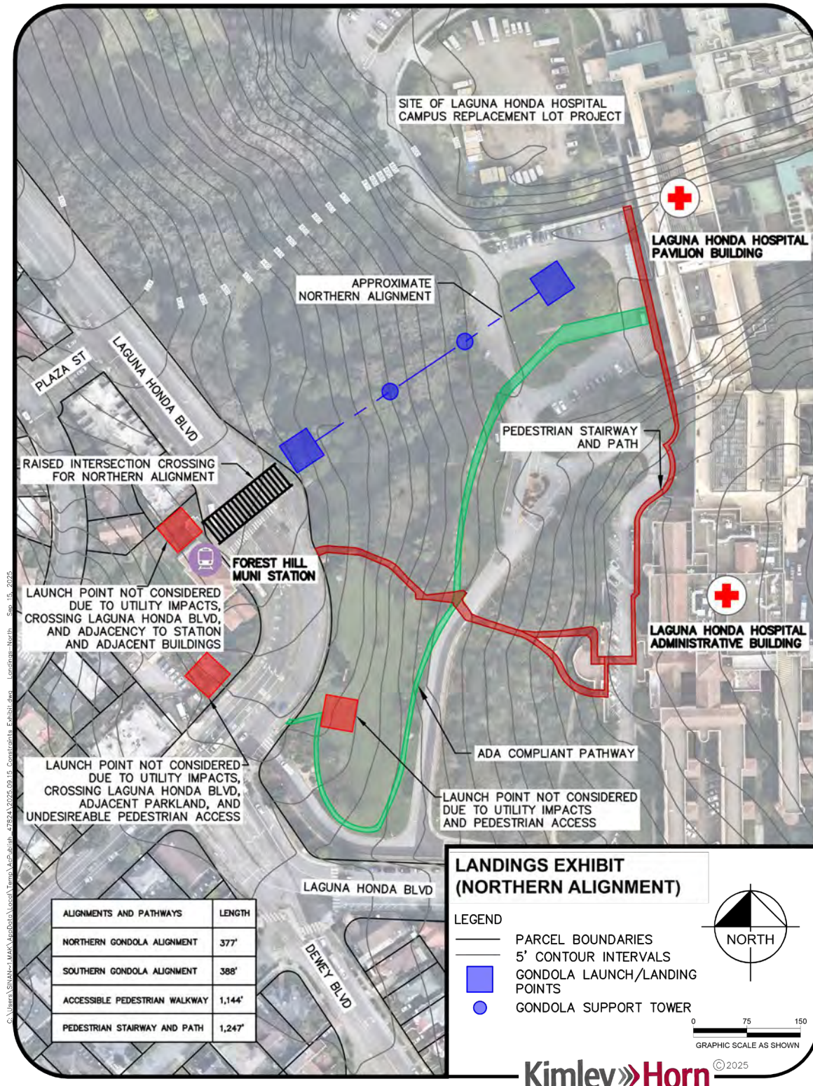
Figure 7-1. Potential Northern Alignment
