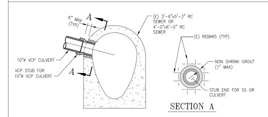
CULVERT CONNECTION DETAIL FOR RC SEWER
