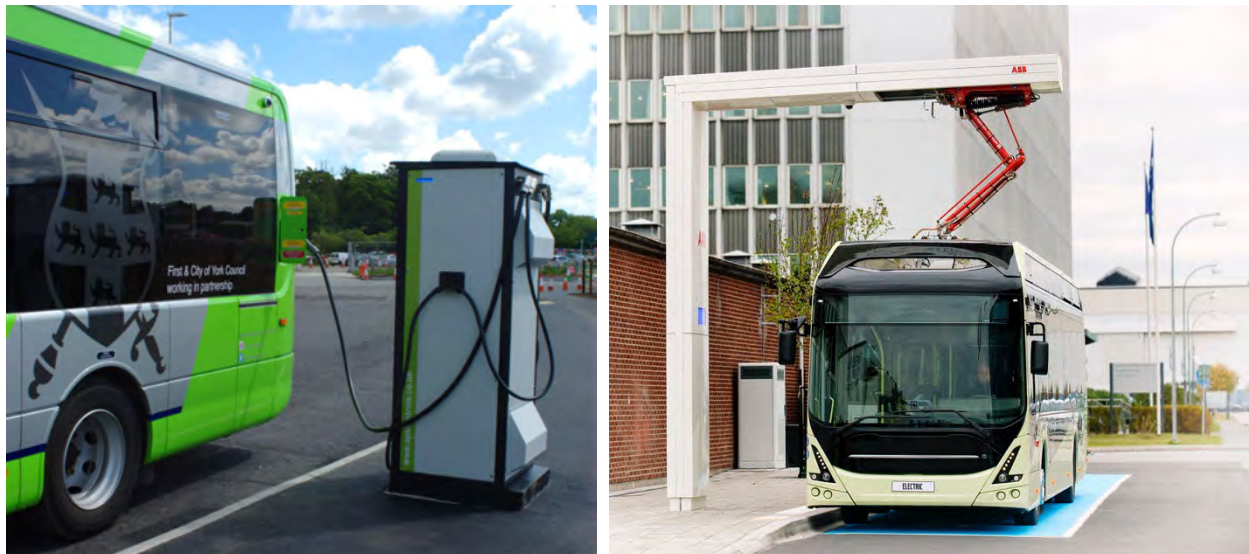
Figure 2-1. Plug-In and Pantograph Charging
