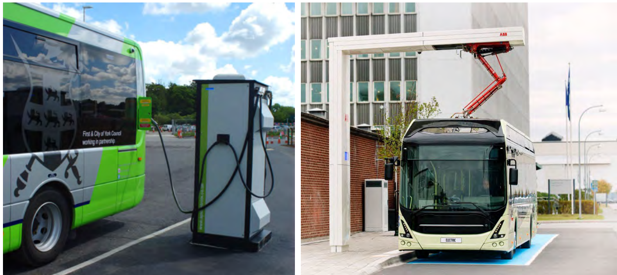
Figure 2-1. Plug-In and Pantograph Charging
