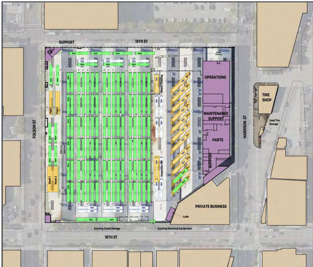
Figure 4-6. Flynn Yard - Existing Conditions (Site Plan)
