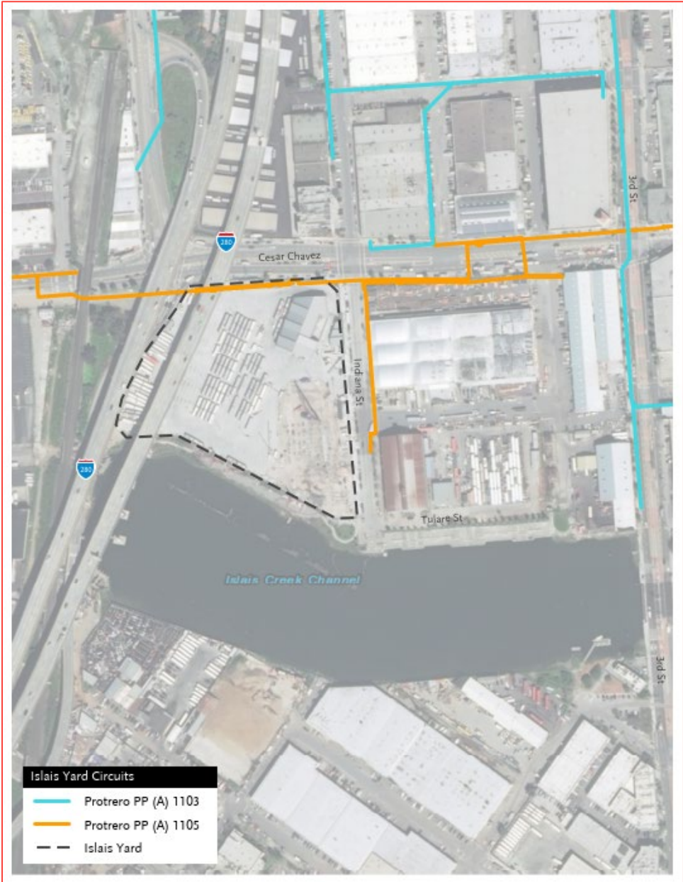
Figure 5-7. Islais Creek Yard – Nearby Circuits
