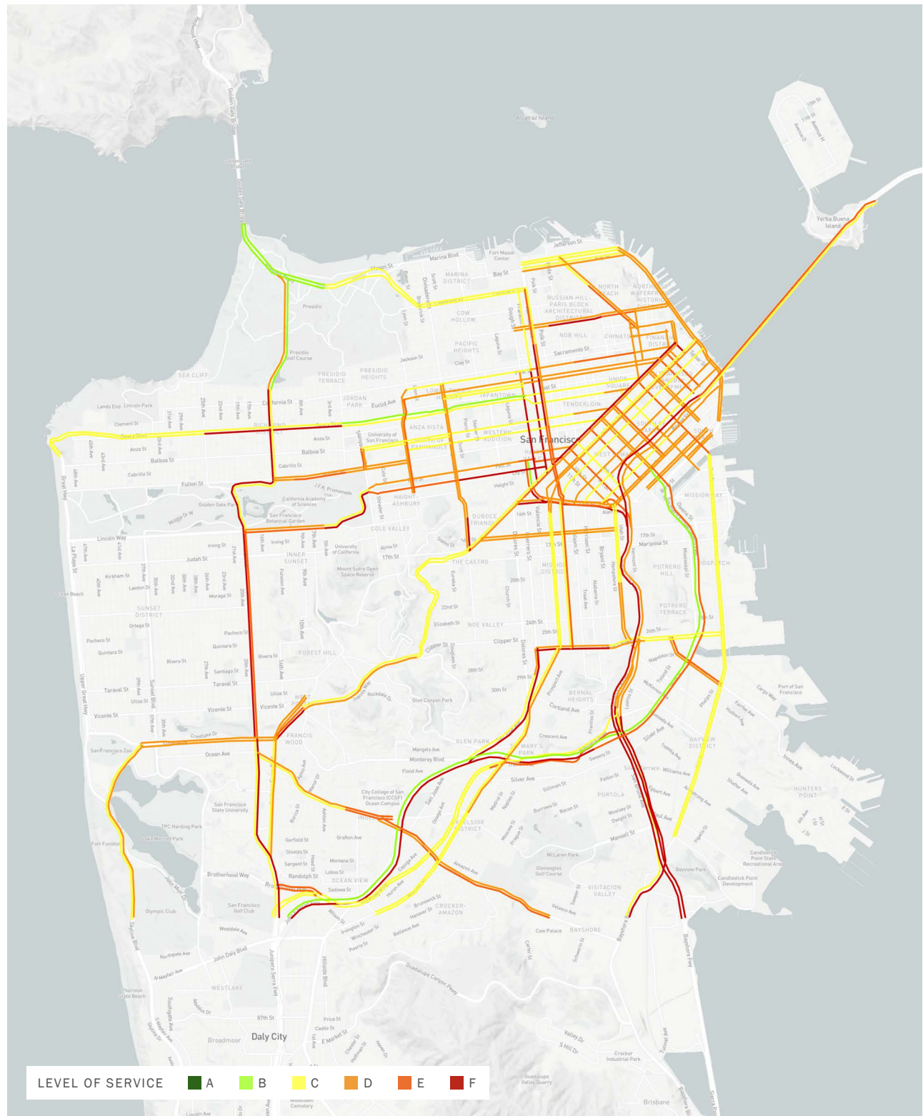
Figure 4-7. 2023 Roadway Buffer Time Index on CMP Network Segments, Weekday AM Peak
