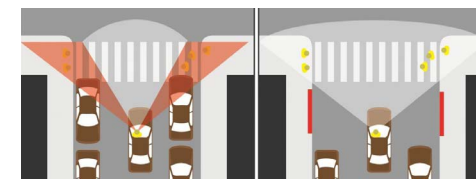
Daylighting at intersection
