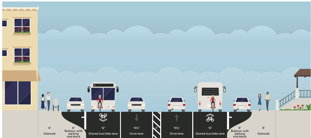
Figure 10. Geneva Transit, Pedestrian, and Bike Improvement Cross Section
