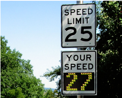
Speed radar signs reduce speeds by 3-9 MPH, and could be used to help educate drivers about new, lower speed limits.
