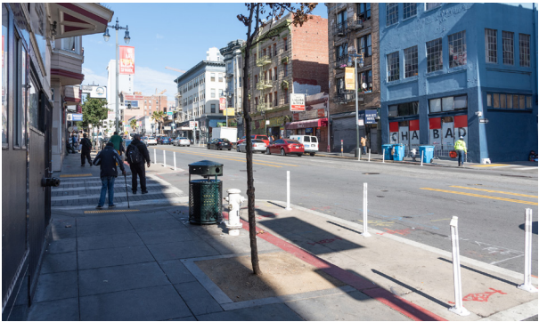
After the ‘Quick Build’ project on 6th Street reduced travel lanes from four to three, 85th percentile speeds went down by 21%.
