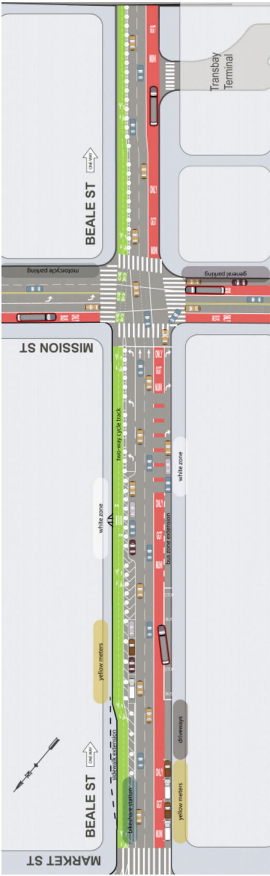
Above: Beale Street with proposed transit-only lane, two-way cycle track between Market and Natoma.
