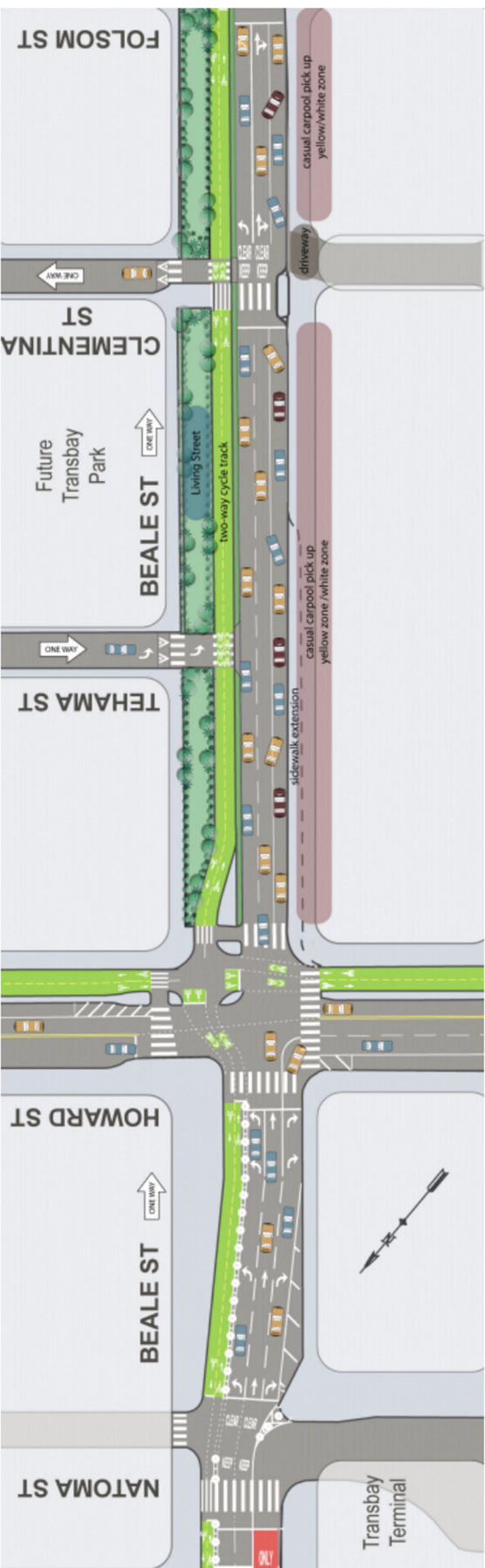
Above: Beale Street with proposed two-way cycle track and sidewalk extensions between Natoma and Folsom streets.
