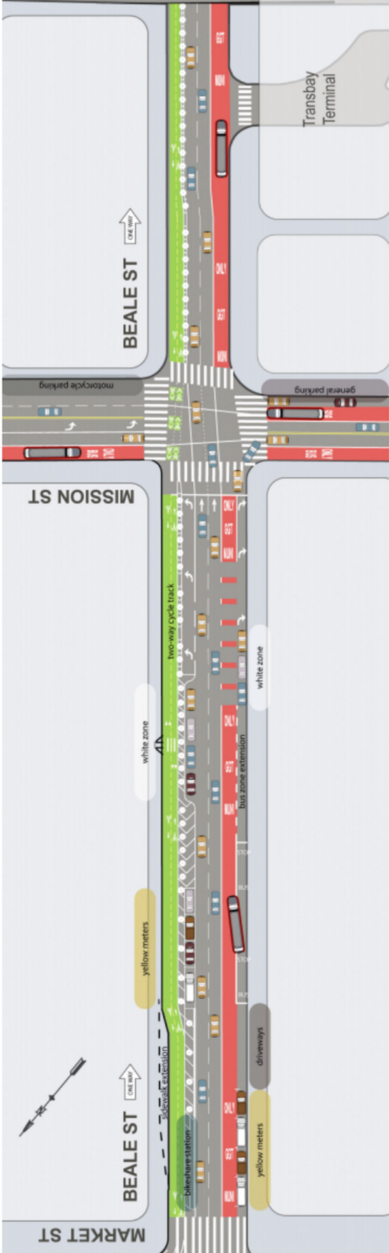
Above: Beale Street with proposed transit-only lane, two-way cycle track between Market and Natoma.
