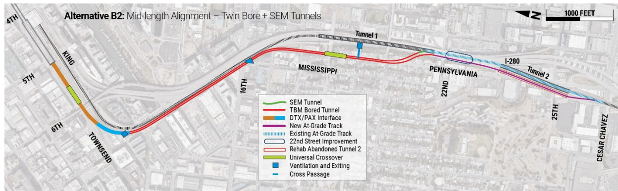
Figure 5-4. Fire/Life Safety Features for Mid-Length Alignment – Twin Bore + SEM Tunnels
