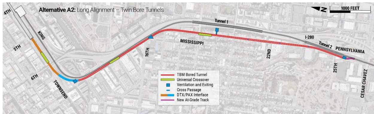
Figure 5-2. Fire/Life Safety Features for Long Alignment – Twin Bore Tunnels
