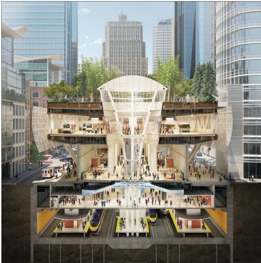
Figure 1.1. Salesforce Transit Center Cross Section
