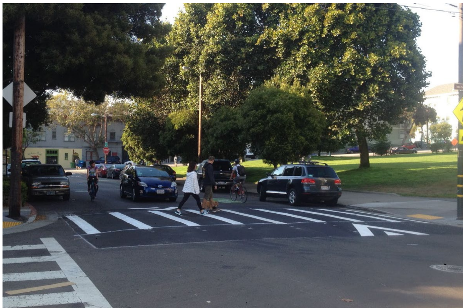
Figure O. Raised crosswalks slow vehicles in areas of significant pedestrian presence
