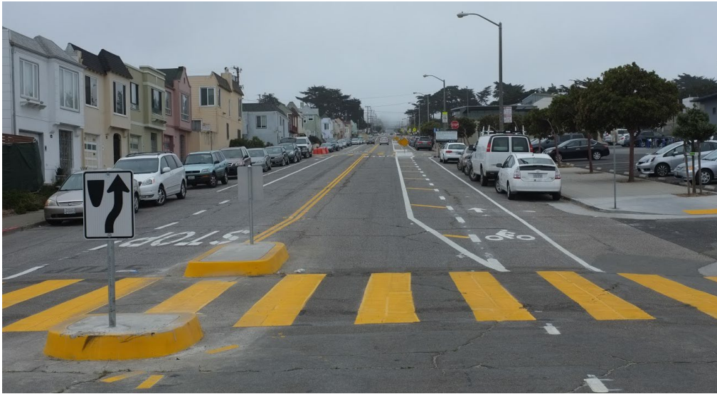
Figure P. Bike lanes designate a portion of the roadway for bicycle use.
