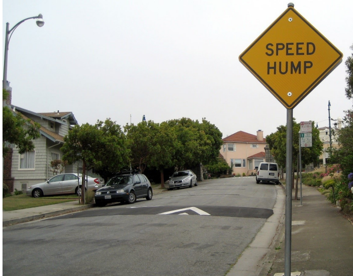
Figure N. Speed humps reduce vehicle speeds
