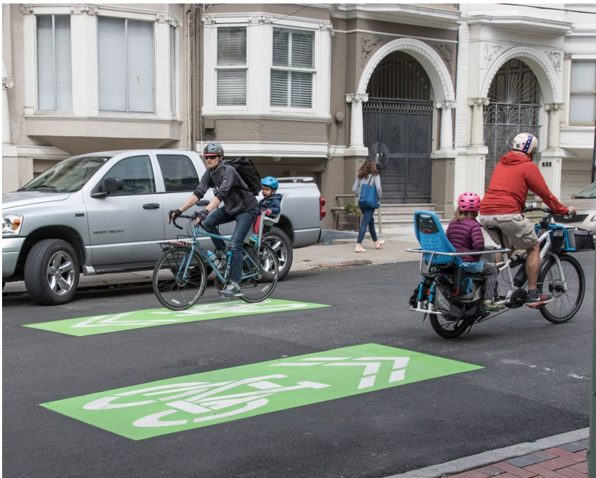
Figure Q. Sharrows indicate the sharing of lanes between bicycles and vehicles.
