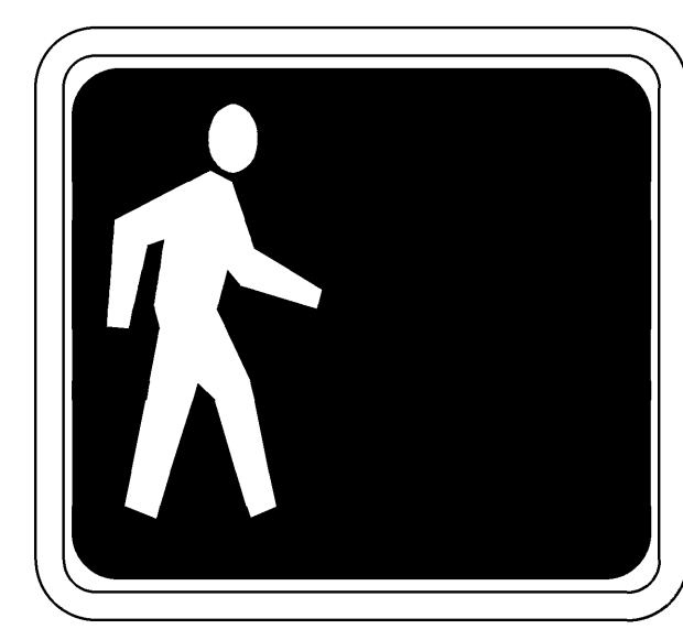
PERSON WALKING INTERVAL FLASHING UPRaised HAND INTERVAL STEADY UPRaised HAND INTERVAL LED COUNTDOWN PEDESTRIAN SIGNAL FACE MODULE DETAIL B
