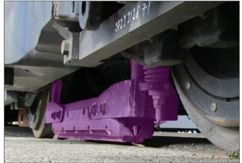
Track brake highlighted in purple. Additional track brakes are being installed on the front and back of the train to reduce flat wheels and improve vehicle availability
