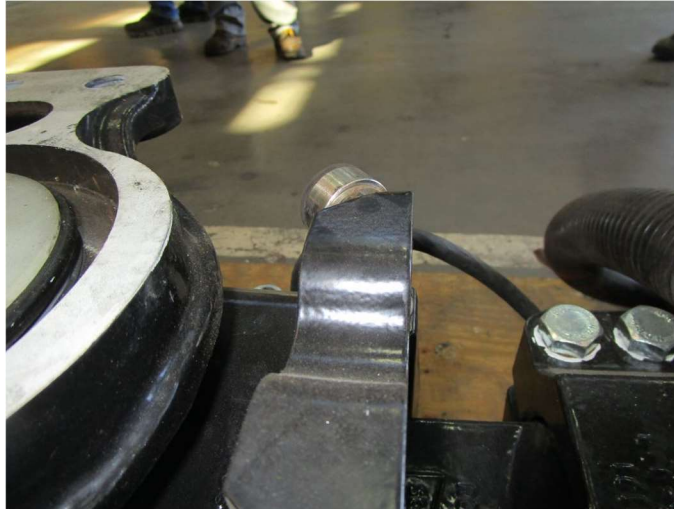
Exhibit 17 – Lateral Stop Bracket Puck Extends 5MM above Bracket
