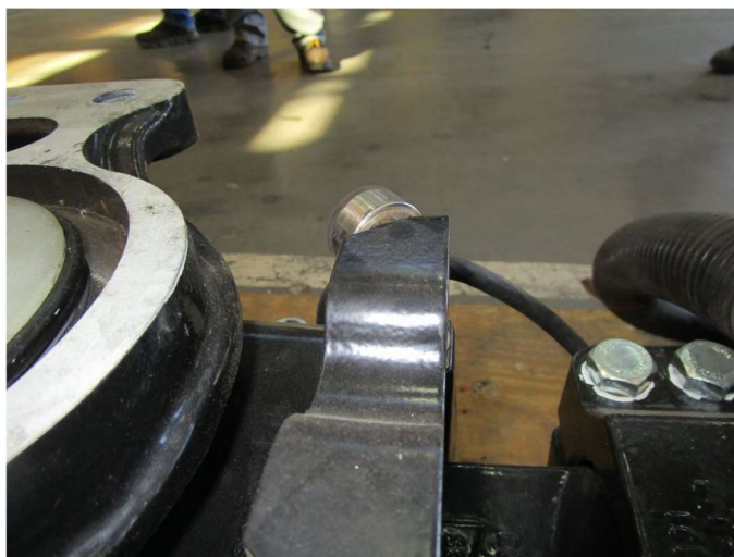
Exhibit 17 – Lateral Stop Bracket Puck Extends 5MM above Bracket
