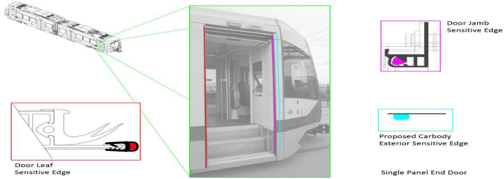
Exhibit 10 – Detail of Sensitive Edge Modification
