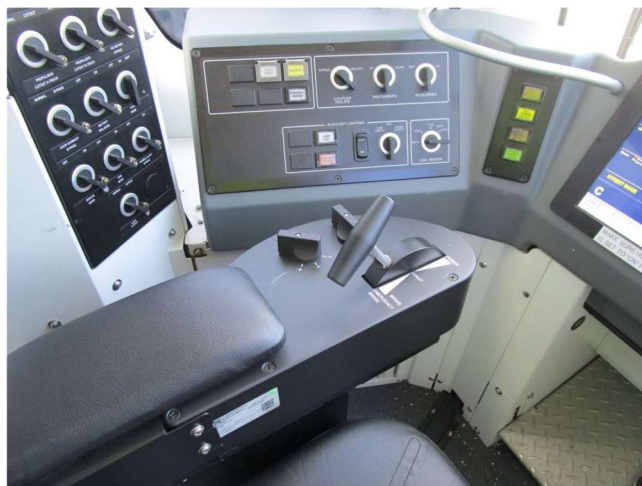
Exhibit 19 – LRV4 ‘T’ Handle in 90 Degree Off Position
