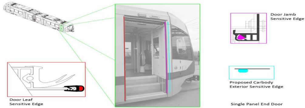
Exhibit 10 – Detail of Sensitive Edge Modification
