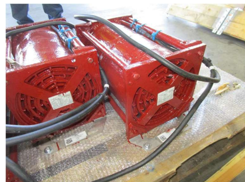
Exhibit 3 – New Design – Brackets extend below bottom of APS for drainage clearance
