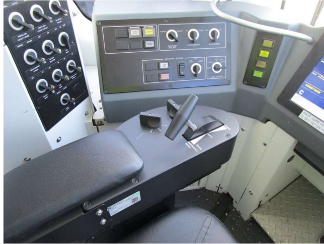
Exhibit 19 – LRV4 ‘T’ Handle in 90 Degree Off Position
