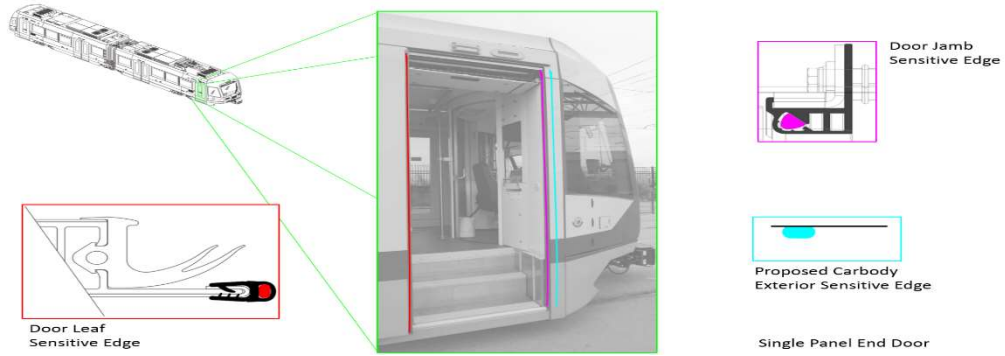
Exhibit 10 – Detail of Sensitive Edge Modification
