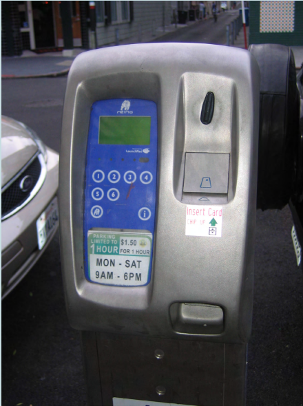
FIGURE 3-15 MULTISPACE PARKING METER
