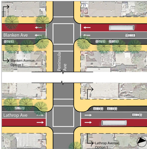
FIGURE 28. PLAN DRAWING OF BLANKEN/LATHROP COUPLET OPTION 1
