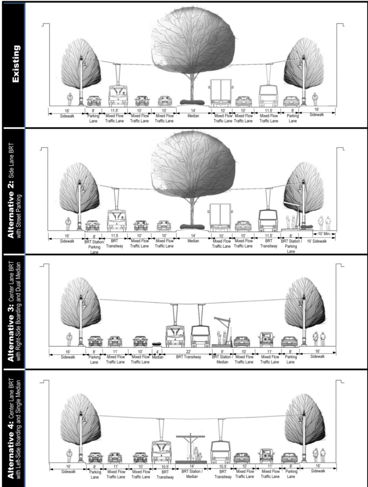
Figure 2-1. Typical Cross Sections of Build Alternatives 2-4
