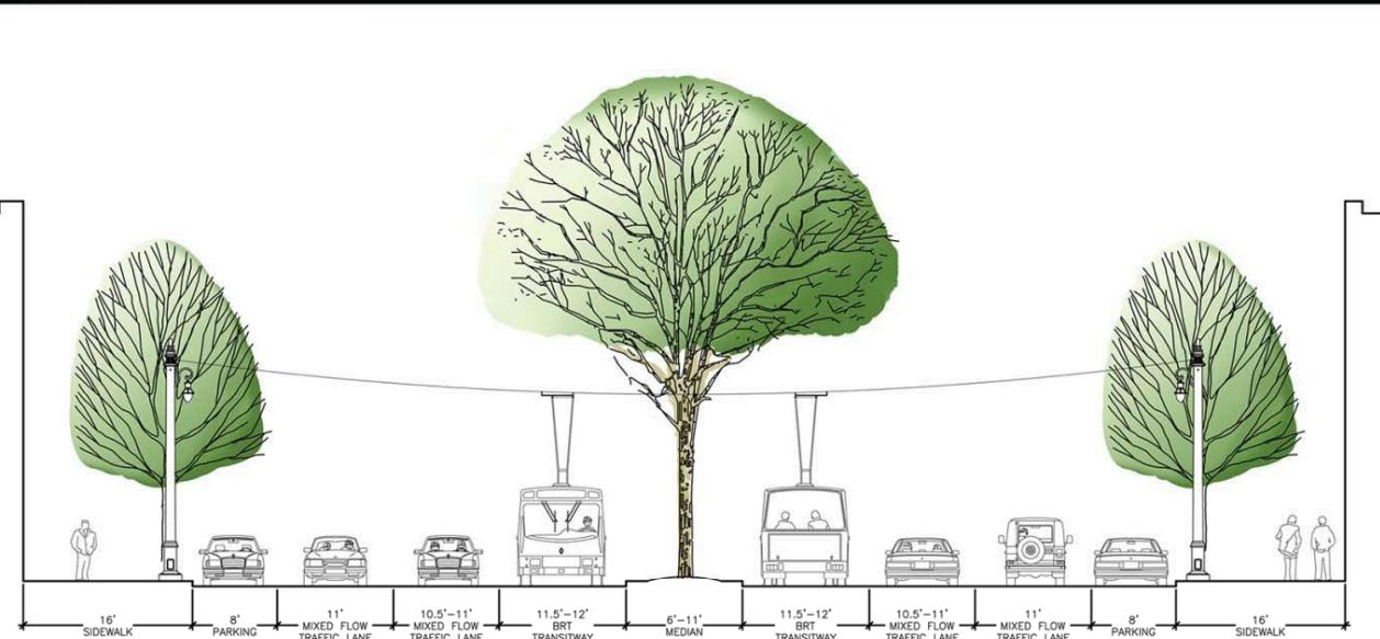
**LPA:** Center Lane BRT with Right-Side Boarding/Single Median and Limited Left Turns
