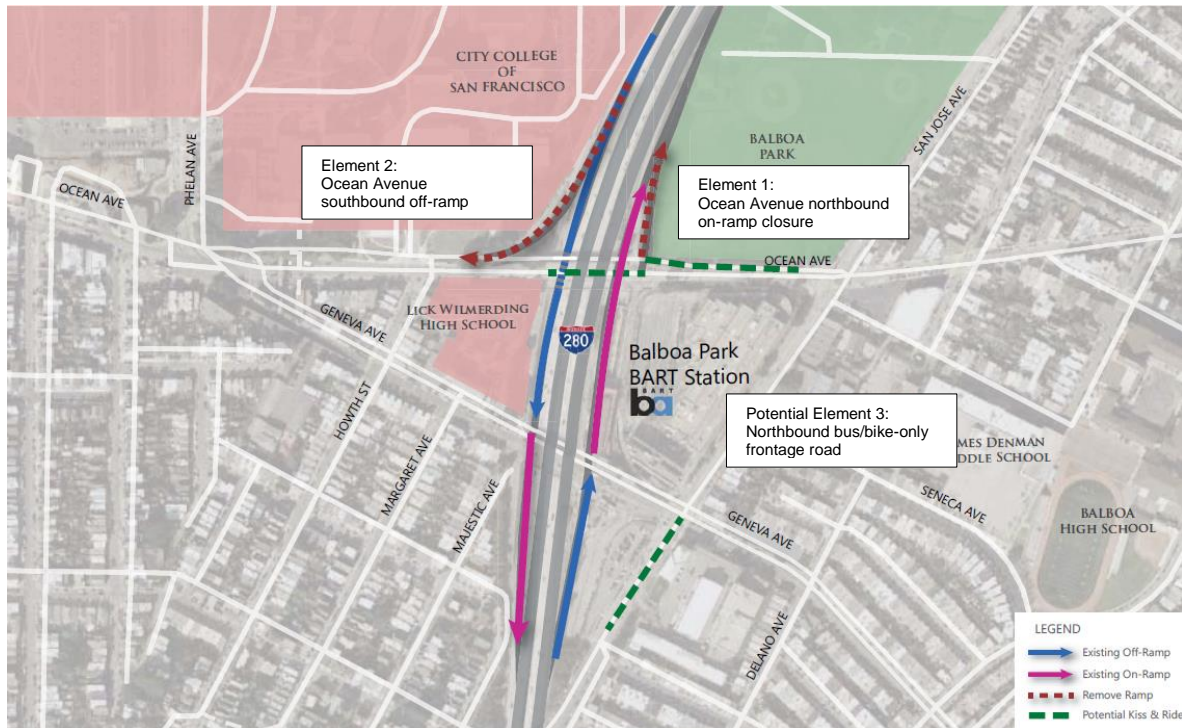
Figure 17: Alternative 2 Consolidated Interchange on Geneva Avenue
