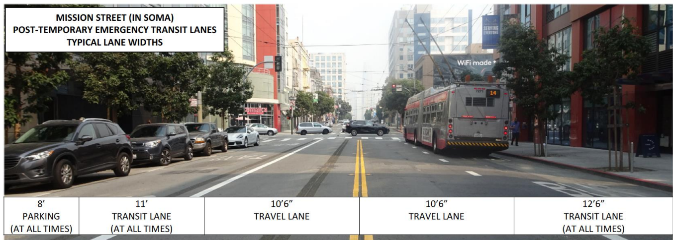
Figure 2: Cross-sections: Previous (above) and Current/Proposed (below)
