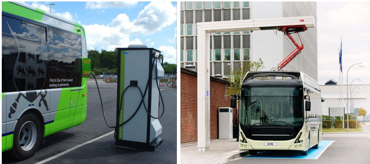
Figure 2-1. Plug-In and Pantograph Charging
